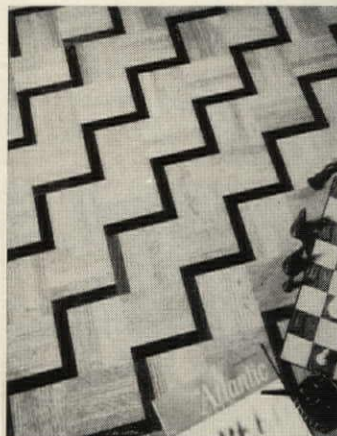
Hardwood flooring comes in 19" x 19" panels, each with sixteen 4 3/4" squares made up of solid square-edged slats. The 5/16"-thick panels are held together with face paper, which is removed after installation. Harris Mfg., Johnson City, Tenn. Circle 209 on Reader Service card
