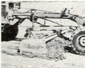
Grading attachment for scrapers cuts off high spots and fills in low spots to make a smooth surface. Blade bowl consists of two sideboards, a spreader bar and a leading cutting edge. It bolts to a standard moldboard. Caterpillar, Peoria, Ill. Circle 222 on Reader Service card
