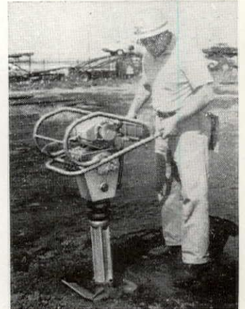
Earth compactor is gasoline powered for one-man operation (no compressor is needed). It delivers seven hundred 1,000-lb. blows per minute. The GT-6 is designed for easy disassembly, maintenance and lubrication. Thor Power Tools, Aurora, Ill. Circle 226 on Reader Service card
