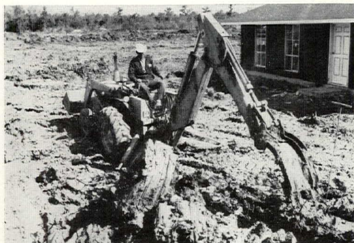
Sideless backhoe bucket digs muck and gumbo and drops material without trouble. Called the Mole Paw, it doesn't clog up with sticky materials as would an ordinary bucket with sides. International Harvester Co., Chicago. (Circle 224 on Reader Service card)
