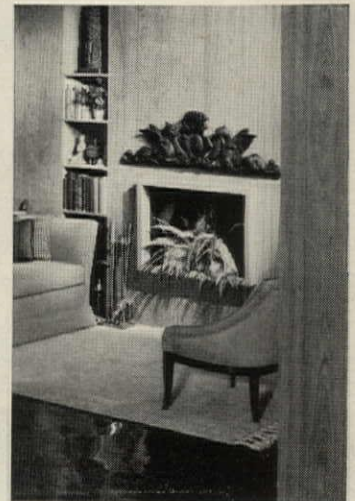
Wood-grain panels have gypsum core and a washable satinelike finish. Six patterns of random-plank panels with three-dimensional grooves are offered in 4' x 8' sheets with matching-color nails. National Gypsum Co., Buffalo, N.Y. Circle 206 on Reader Service card
