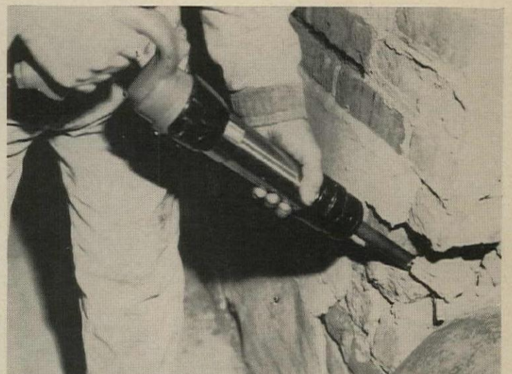
Air-operated chipping hammers are available with 1", 2" and 4" strokes. All units are less than 20" long and weigh 17 1/2 lbs. The hammers have an air cushion design that is said to eliminate shock. Thor Power Tool Co., Aurora, Ill. Circle 234 on Reader Service card.
