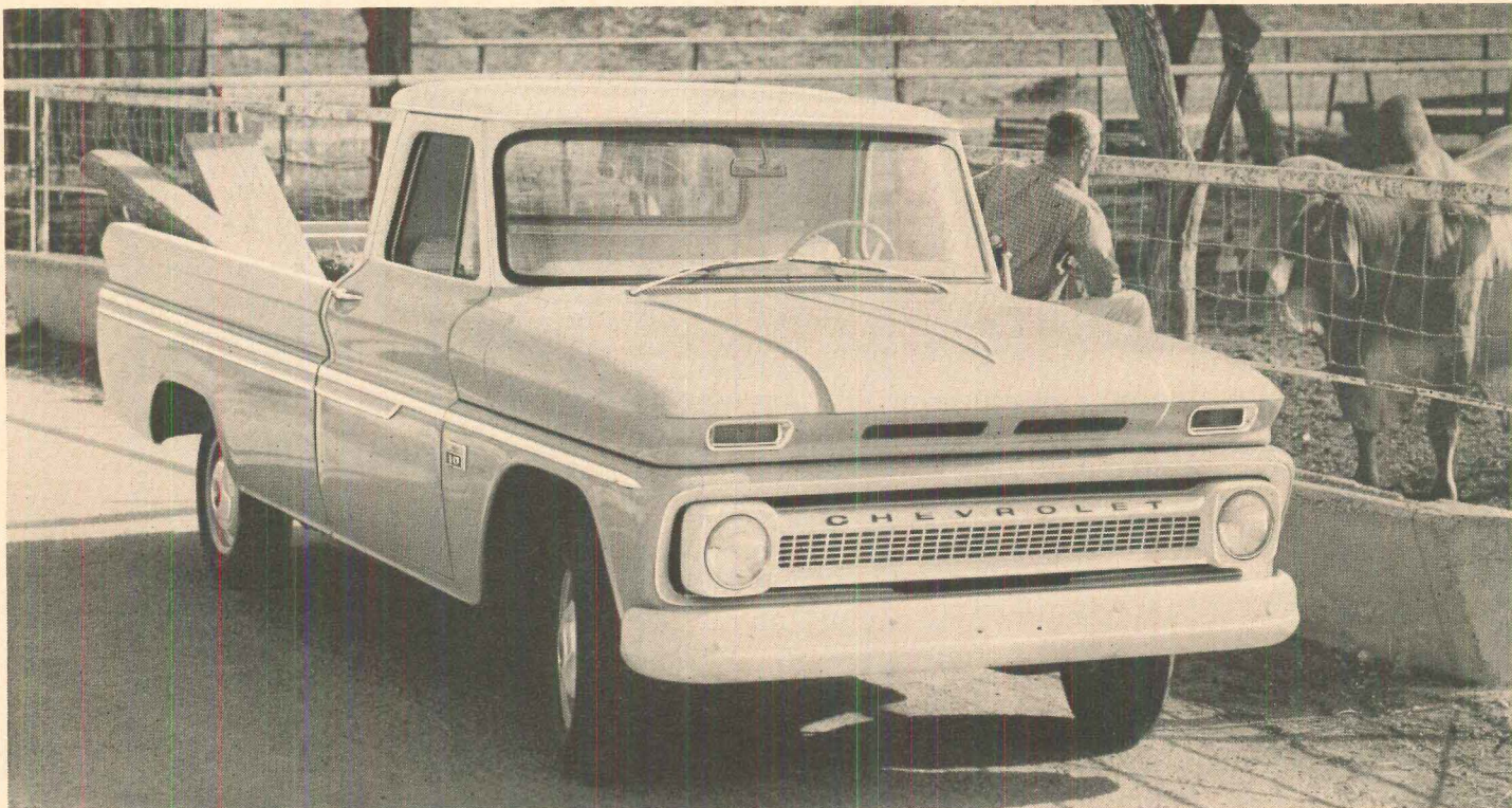
3 FLEETSIDE MODELS —Trim-lined Fleetside bodies are offered in 6½-ft. and 8-ft. lengths. Double-wall lower body side panels keep cargo dents from marring exterior appearance, and tough wood floor planking is joined by full-length steel skid strips. Maximum GVW ratings from 5,000 to 7,500 pounds.
