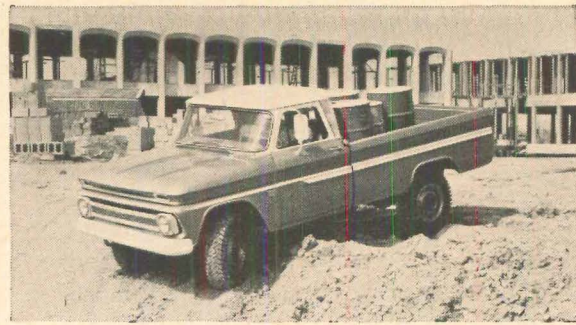
6 FOUR-WHEEL-DRIVE MODELS —Go-anywhere traction is offered with either Fleetside or Stepside bodies in 6½-ft. or 8-ft. lengths. Extra rugged chassis and drive line includes 2-speed transfer case. Maximum GVW ratings from 5,600 to 7,600 pounds.
