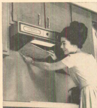
Ducted hood features an easy-to-remove aluminum mesh filter and an extra-wide enclosed light. Comes in several colors with a 200-cfm impeller-type fan, and may be ducted horizontally or vertically through a 3¼"x10" duct. Nutone, Cincinnati, Ohio. Circle 316 on Reader Service card
