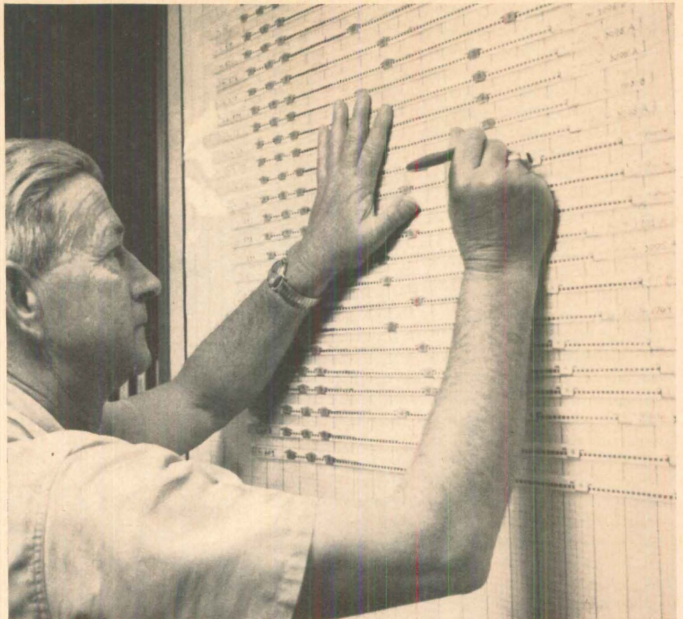
PROGRESS CHARTS , updated by superintendents, are based on detailed planning networks like the one below (only about half is shown), which allows 74 days for a one-story house.
