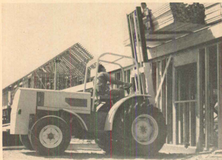
Fork-lift truck designed especially for rough terrain can be safely towed at highway speeds up to 70 mph. Lift rating is 5,000 and 6,000 lbs. at 24" load centers. Standard masts lift to 21', optional masts to 30'6". Scotsman, Tulsa, Okla. Circle 250 on Reader Service card
