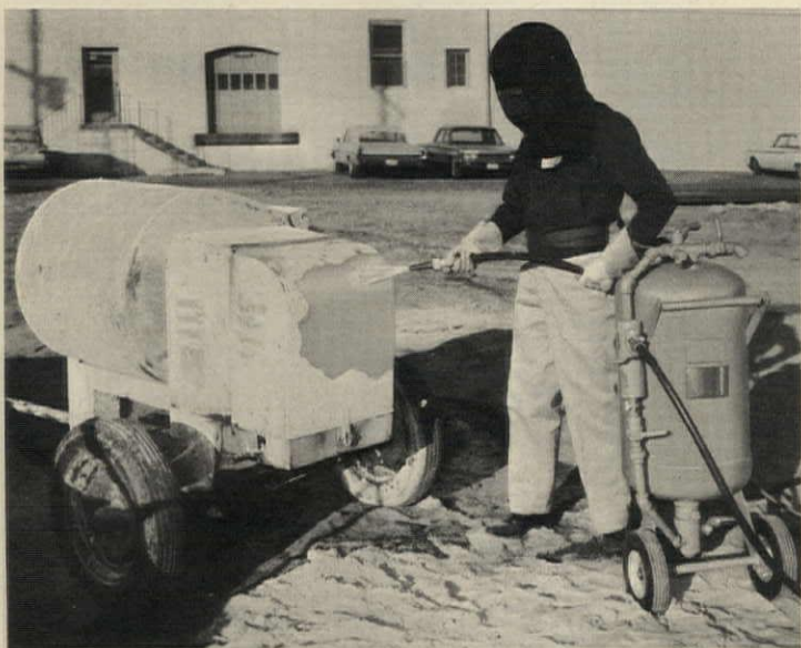
Portable pressure blaster —for removing paint, rust and corrosion—is filled with abrasive and hooked up to air supply. Agitator keeps abrasive free-flowing. Equipment: 20' hose, nozzle assortment, filler funnel, hood. Inland, Omaha. Circle 265 on Reader Service card
