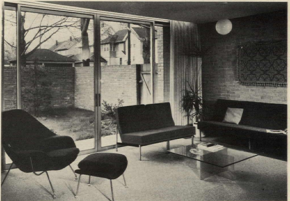
FULL-GLASS WALL in front of living room opens to walled garden. Wall is high enough for privacy, low enough to avoid closed-in feeling.
