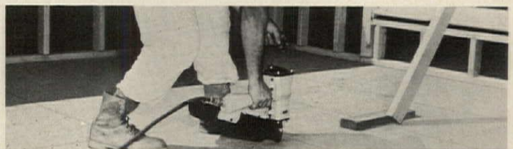
Pneumatic nailer drives a range of nails from 6d common through 16d sinkers. It can be operated with one hand and has a built-in safety feature: operator must perform two separate actions to drive a nail. Duo-Fast, Franklin Park, Ill. Circle 277 on Reader Service card
