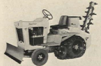
Half-track trencher —also a tractor—steers through the front wheels but can also steer itself when trenching. It digs hydraulically, from 4" to 14" wide, up to 58" deep, and runs on an 18-hp gasoline engine. Arps, New Holstein, Wis. Circle 271 on Reader Service card
