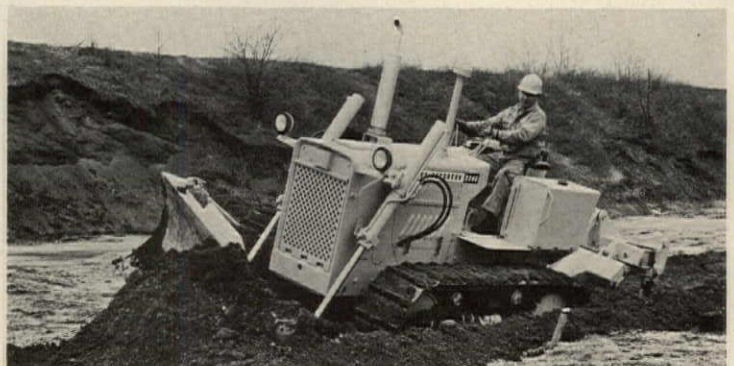
Crawler tractor in the 75-hp class has a 302-cu.-in diesel engine and a hydraulic reversing transmission. Two models available: a dozer (shown) and a loader with 1 1/2-cu.-yd. capacity bucket. Massey-Ferguson, Des Moines. Circle 276 on Reader Service card
