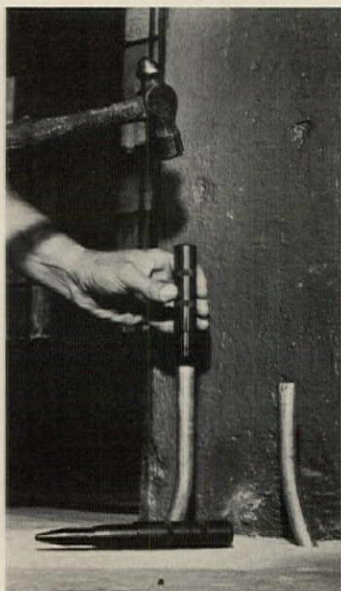
Sizing tool re-shapes floor stub-ups or any 1/2" and 3/4" thin-wall conduit accidentally damaged during installation. It can also be used to make slight bends in conduit ends for final alignment after installation. Ridge Tool, Elyria, Ohio.
