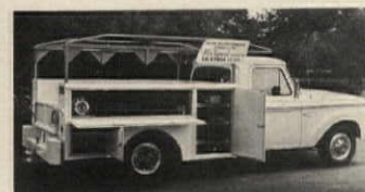
Utility body designed especially for building contractors features outside tool compartments fitted with removable shelves and adjustable bins. Compartments are protected against vandalism and theft by slam-action locks. Reading Body, Reading, Pa. Circle 264 on Reader Service card
