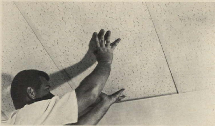
Fissured ceiling panels are \frac{5}{8} " thick, rated Class A (incombustible), and weigh about .60 lbs. per sq. ft. Available in two sizes—2'x2' and 2'x4'—with a noise-reduction coefficient of .80. Celotex, Tampa, Fla. Circle 225 on Reader Service card
