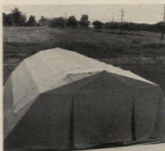
Relocatable dome built of lightweight galvanized-steel tubing is covered by nylon-reinforced vinyl with translucent sections to let in daylight. It spans 30' to 45', can be any length, and bolts together. Versadome, Montgomeryville, Pa. Circle 268 on Reader Service card
