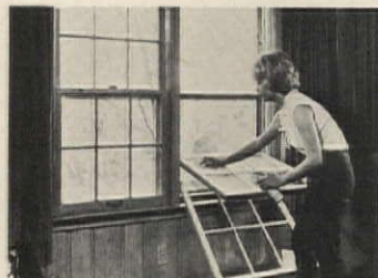
Tilt window allows removal of both top and bottom sash, yet air infiltration is claimed to be just 50% of the allowable standard. Each sash is balanced on both sides. Head, sill and check-rails are weathersealed. R.O.W., Ferndale, Mich. Circle 361 on Reader Service card
