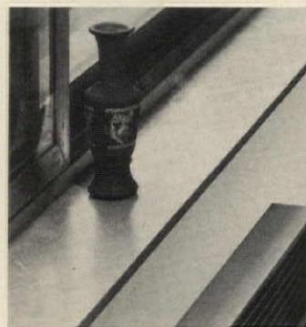
Plastic window sill comes in marbles ( above ), woodgrains and solid colors. It can be milled, drilled and sawed with ordinary woodworking tools. Standard dimensions: \frac{1}{2} " thick; 4\frac{1}{2} " to 9\frac{1}{2} " wide; 3' to 12' long. Kenmore, Lowell, Mass.
