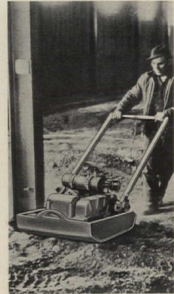
Vibratory compactor —powered by an air-cooled, 8-hp gasoline engine—covers areas of up to 10,500 sq. ft. per working hour and delivers an impact force of 6,300 lbs. Base plate measures 32"x24" and is ½" thick. Wacker, Milwaukee. Circle 266 on Reader Service card
