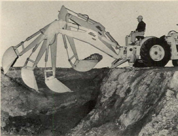
Automated backhoe in three sizes—10', 13' and 15'—speeds digging by allowing the operator to fill the bucket by pulling one lever instead of the three separate levers used in standard backhoes. Ford, Birmingham, Mich. Circle 281 on Reader Service card
