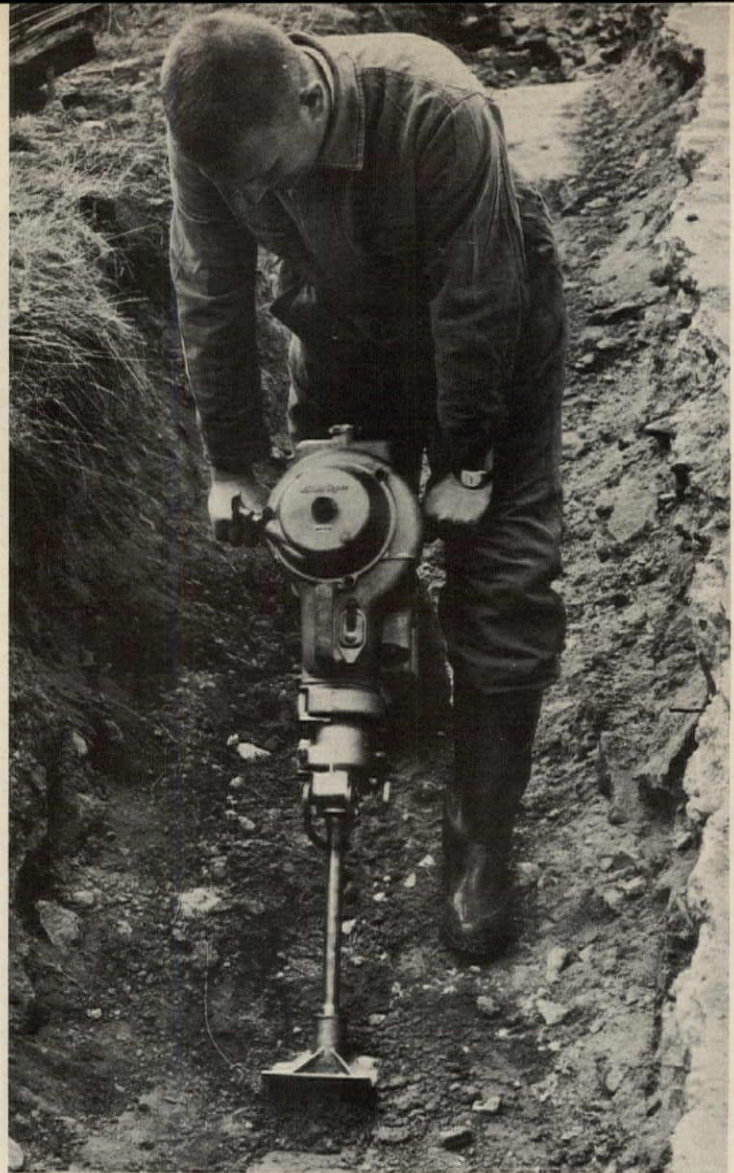
Drill/breaker offers an 8"x8" rammer pad set at a 60° angle to the rammer stem. The design makes the tool move when ramming—an advantage for working on backfilled cable ducts and similar jobs. Weight: 56 lbs. Atlas, Hackensack, N.J. Circle 280 on Reader Service card
