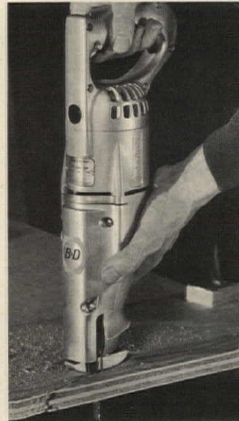
Two-speed sabre saw cuts soft wood, plastic and composition at 2200 strokes per minute; and cuts hardwood, mild steel and conduit at 1100 strokes per minute. Serrated blade clamp gives maximum holding power. Black & Decker, Towson, Md. Circle 265 on Reader Service card
