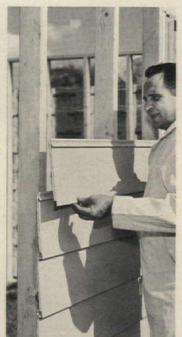
Sandwich-panel siding combines factory-enameled aluminum, polystyrene insulating foam, aluminum foil and kraft paper. Panels can be applied directly to studs, and are vented by 1/8" holes on 17" centers. Also, Akron, Ohio. Circle 244 on Reader Service card
