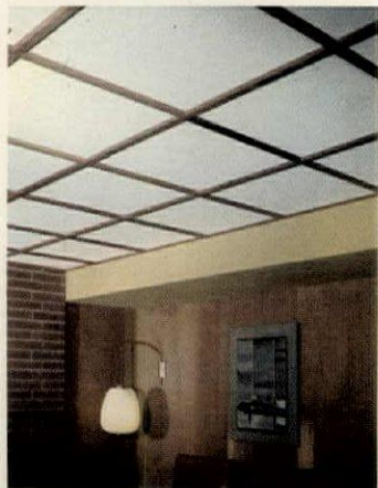
Easy-to-install ceiling needs no backing or suspension system: Redwood runners are nailed directly to joists, and then 2'x2' or 2'x4' lay-in panels—either acoustical board or light diffusers—slide into place. Cross members conceal joints. Simpson, Seattle. Circle 200 on Reader Service card
