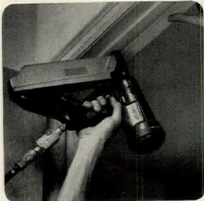
Finish and Brad Nailers drive finish nails and brads 5/8" to 2" long.
