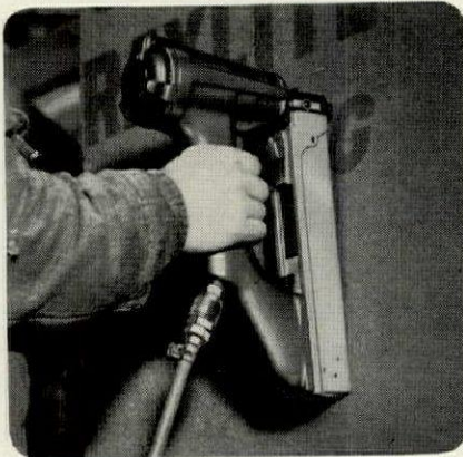
The Staple Nailer drives heavy, coated Duo-Fast Staples up to 2" long.
