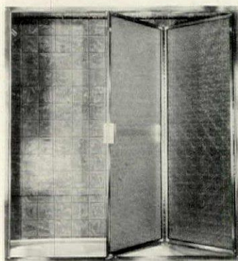
Folding tub enclosure that permits almost total accessibility to the tub area is offered in hammered frosted glass (photo) or plastic laminate. Designed for standard 5' tubs, enclosure is 58" high, fits 57" to 59" openings. Theodore Efron, Chicago. Circle 215 on Reader Service card
