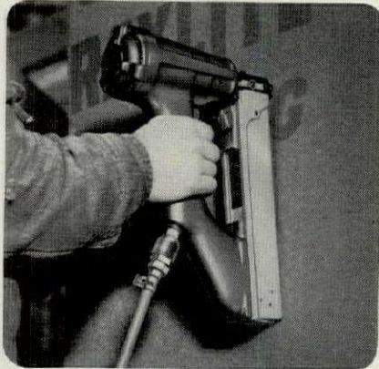
The Staple Nailer drives heavy, coated Duo-Fast Staples up to 2" long.
