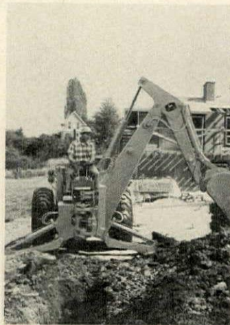
Backhoe for use with manufacturer's JD300 and JD400 loaders has 2,000-lb. vertical load-lifting capacity; 6,750-lb. digging force; and 180° arc of swing. Nine buckets range in capacity from 1.6 to 7.2 cu. ft. Deere & Co., Moline, Ill.
