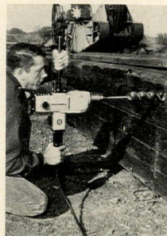
Heavy-duty drill for big-hole drilling in metal or wood is one of 12 models with 12- or 15-amp motors and choice of four speeds. A multi-position handle rotates 90° to give maximum leverage for drilling or reaming large holes. Rockwell, Pittsburgh.
