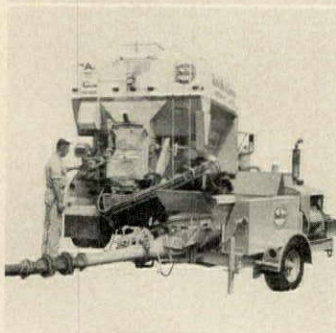
Small concrete pump will move from 14 to 16 cu. yds. per hour, can be towed easily behind a pickup truck. Manufacturer suggests that pump's lower price makes it feasible to use two at large pours as insurance against the delays caused by plugs. Pump is shown at left being supplied by concrete mixer truck (H&H, Oct.). National Concrete Machinery, Lancaster, Pa.
