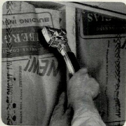
Hammer Tacker drives \frac{1}{4} " to \frac{5}{16} " staples as fast as you can swing it.
