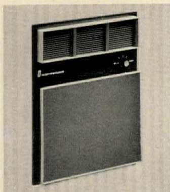
In-the-wall heater works much like electric hot water baseboard heaters, is available in 120- and 240-volt models and has 1,000-watt capacity. Unit requires 4" depth in masonry wall, projects only 1¼". International Oil Burner, St. Louis. Circle 232 on Reader Service card
