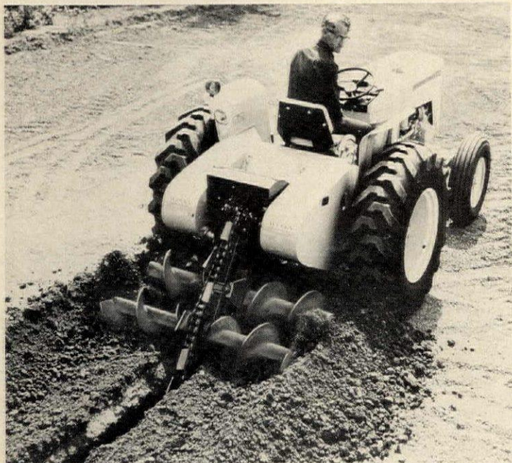
Hydraulic trencher can dig smooth trenches from 6" to 14" wide and up to 6' deep at speeds up to 900 ft. per hour, depending on soil conditions. Hydraulic control assembly is a complete, removable unit. International Harvester, Chicago. Circle 228 on Reader Service card
