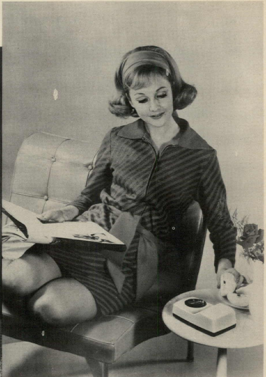
ELECTRONIC THERMOSTAT is wireless, completely portable. It sends signals to a responder installed on or near the furnace or air conditioner. Because it can regulate temperature from any spot in the house, it can be used to correct an uneven system or to simulate a multi-zone system. Kimco Laboratories, Brooklyn, N.Y. Circle 209
