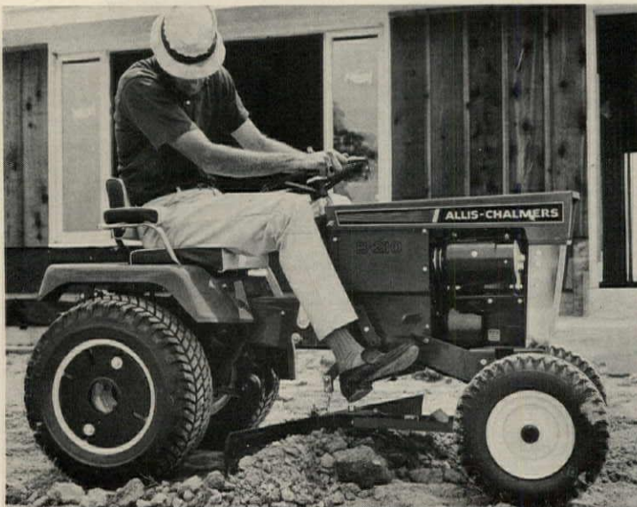
Landscaping tractor features floating axles that follow ground contours, a differential that applies continuous torque to both rear wheels. Attachments include grader shown, plus mowers, trenchers, etc. Allis-Chalmers, Milwaukee, Wis. Circle 268 on Reader Service card
