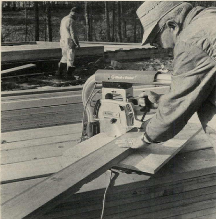
Radial arm saw weighs 58 lbs.; light enough for on-the-job work, tough enough to cut a 2x6 as shown. It will also bevel, rip, or miter. A 2-hp motor pushes 8" blade through 2 7/8"-deep cuts. Black & Decker, Towson, Md. Circle 267 on Reader Service card
