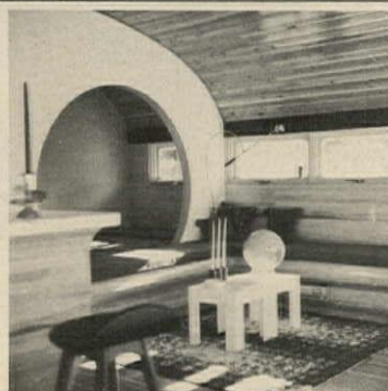
Boat-like interior has contoured ceiling and counter, circular windows, and alcove (lower right) with pull-out bed. U.S. prototype of deluxe model, shown here, had fir and mahogany interior finish, but interiors of production models will be wood-grained fiberglass. Exteriors, also fiberglass, are available in a choice of colors.
