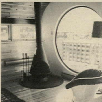
Boat-like interior has contoured ceiling and counter, circular windows, and alcove (lower right) with pull-out bed. U.S. prototype of deluxe model, shown here, had fir and mahogany interior finish, but interiors of production models will be wood-grained fiberglass. Exteriors, also fiberglass, are available in a choice of colors.
