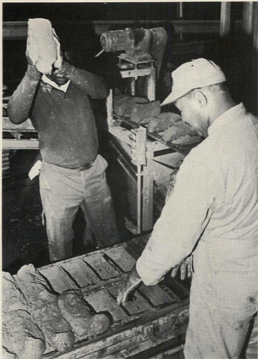
Throwing station is where slugs of raw clay are plopped into wooden mold boxes by hand.
