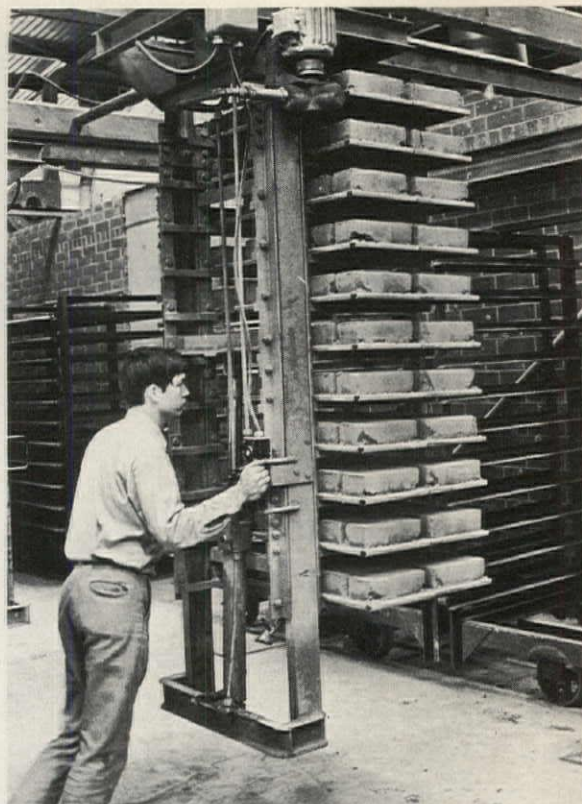
Pallets of bricks are first moved by rack car to drying chamber.
