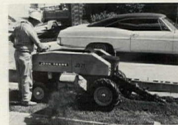
14-horsepower trencher has 4-cycle, air cooled, cast iron engine, hydraulic transmission with oil bath lubrication, and selective differential lock. Features also include matched 4-belt digging drive, tubular booms in 2 1/2', 4 1/2', 4 1/2', and 5 1/2' lengths, with hardened chain guides and spring-loaded boom-end sprocket. Cutter chain strength: 46,000 lbs. John Deere, Moline, Ill.
