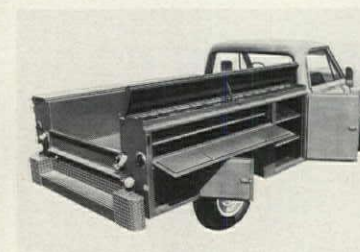
Utility bodies with two extra top-opening compartments are part of a line of 18 low-profile and standard models for chassis from 1/2 to 1 ton. A slide-fold brace engages automatically to hold each lid in open position. 15 removable bin dividers, adjustable on 1" centers, equip each compartment. Units are only 1 1/4" higher than standard for good visibility. Reading, Reading, Pa.
