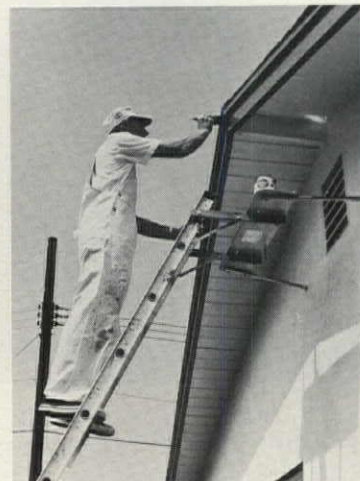
Standoff attachment for extension ladders also includes 236-sq.-in. shelf that holds up to 70 lbs. of tools, paints, or materials. When retracted, shelf supports make handy brackets for hanging cans, rags, etc. Fits any wood or metal extension ladder and can be adjusted to hold workman 18" to 30" from vertical surface. Simple adjustment makes it possible to straddle outside corners of buildings. Wokasch, Whittier, Calif.
