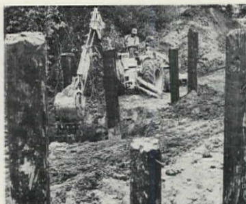
Extending backhoe makes possible working close to walls, fences, or among obstructions, as above. Eliminates need for extensive turning and maneuvering by hydraulically reaching the boom through narrow openings and over obstacles. J.I. Case, Racine, Wis.
