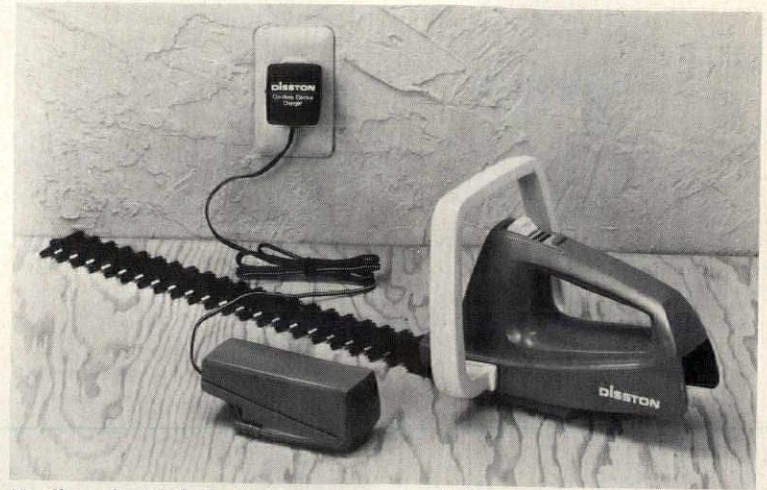
Cordless electric hedge trimmer , to maintain large areas, features an interchangeable battery pack. The tool will deliver 2,200 strokes per minute with its double-edged blade, for up to 45 minutes on a single battery charge. Freshly charged batteries may be inserted on the spot for additional trim time. Disston, Pittsburgh, Pa. CIRCLE 257 ON READER SERVICE CARD.
