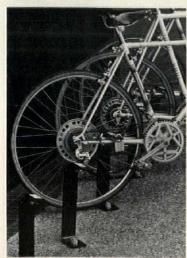
Anti-theft bicycle rack houses and secures bike frame and rear wheel assembly. Constructed of one-piece 3/8" formed steel plate with a protective coating, the rack is anchored to the ground with vandalproof bolt. Inconspicuous units can be arranged to insure maximum use of space. Rally, Mill Valley, Calif.
