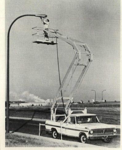
Articulating boom platform lift moves horizontally as well as vertically. The 72"x30" platform has a 500 lb. capacity and a maximum height of 32'. Controls can be operated from a master station, from the platform or from the ground. Up-Mobile, Sacramento, Calif. CIRCLE 254 ON READER SERVICE CARD.
