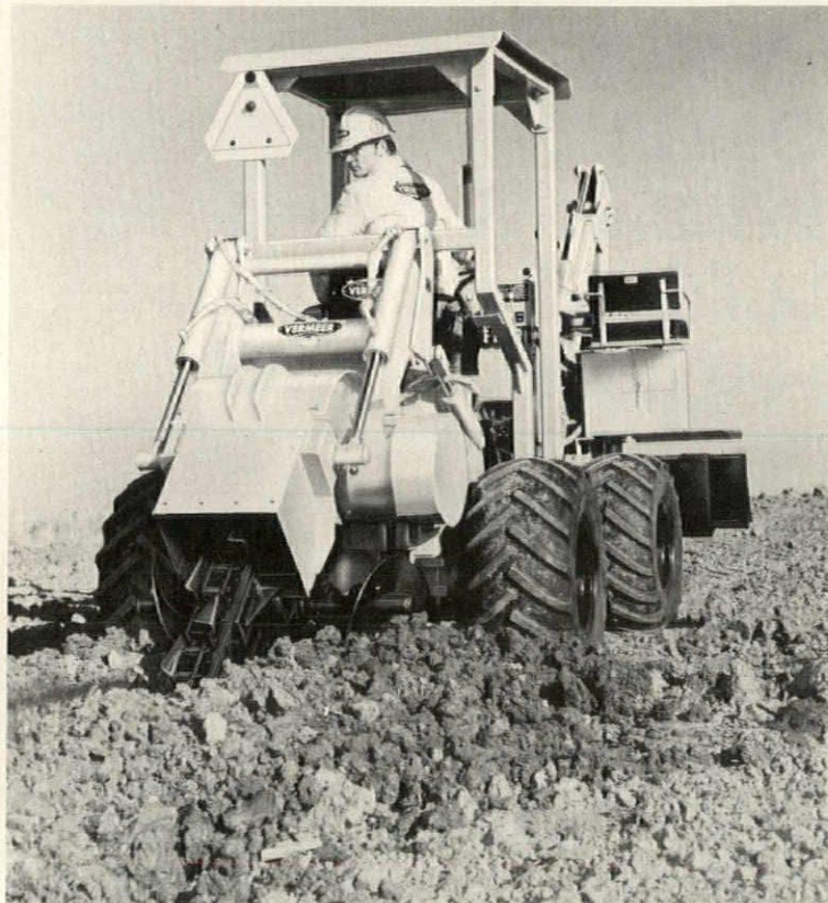
Versatile trencher, "M-440", is capable of performing a variety of dirt-handling tasks. Equipped with a trencher, backhoe and dozer blade attachments, the unit is powered by a liquid-cooled Ford engine. Vehicle has 4-wheel drive, power steering, center pivot articulation and three tire sizes for various traction needs. Vermeer, Pella, Iowa. CIRCLE 260 ON READER SERVICE CARD
