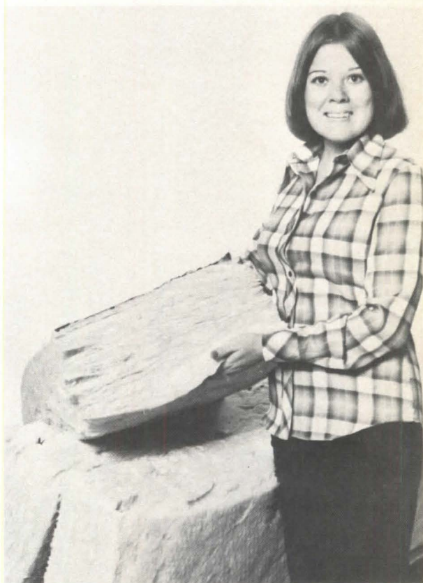
Fiber glass insulation batt (above) is rated R-30. The 8½"-thick batt is available in 15" and 23" widths and 4' lengths. Unit comes either unfaced or kraft faced and is compression packaged to facilitate storage and delivery. Insulation meets present standards. Johns-Manville, Denver, CO. Circle 253 on reader service card
