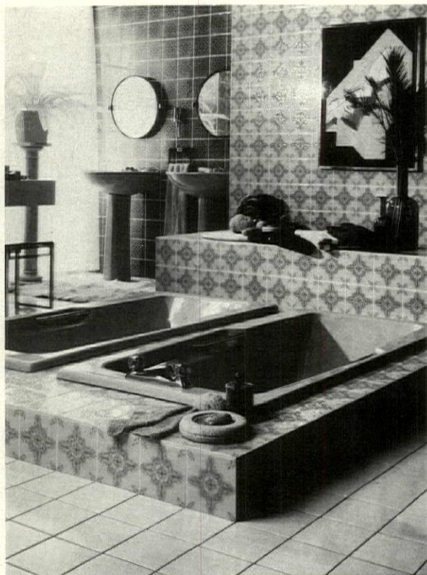
Ceramic wall tiles, "Cristal" (above), can be easily applied directly over old ceramic tiles or other smooth surfaces. Tiles with adhesive backing need no special preparation or equipment for installation. H. R. Johnson, Keyport, NJ. Circle 211 on reader service card
