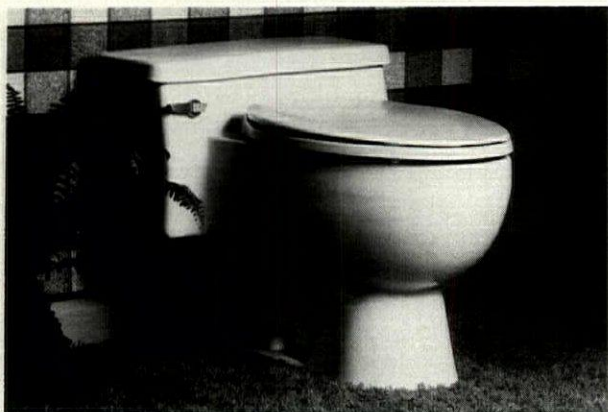
One-piece water-saving toilet, "Silhouette Conservor II" (above), uses only 3½ gallons of water per flush. Unit, available in a choice of colors, has a round-front bowl and a positive non-overflow feature. Briggs, Tampa, FL. Circle 200 on reader service card
