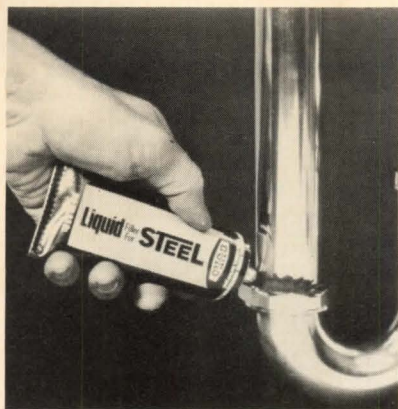
Ready-mixed liquid steel (above) seals holes in gutters, downspouts, radiators and pipes. Layers should average around 1/8" thick; hardening time is 3 to 4 hours. Woodhill Permatex, Cleveland, OH. Circle 209 on reader service card
