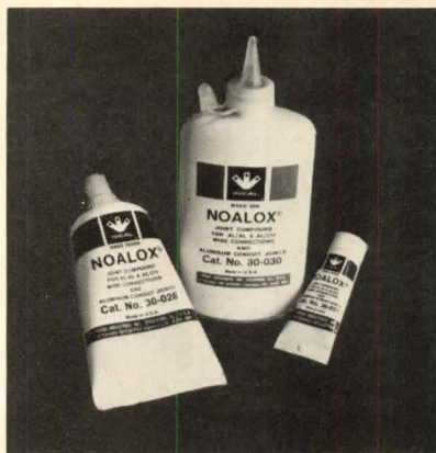
Noalox® anti-oxidant (above) improves conductivity with aluminum wire. Compound is said to cut through aluminum oxide, providing inter-strand and inter-conductor current paths. Ideal, Sycamore, IL. Circle 207 on reader service card
