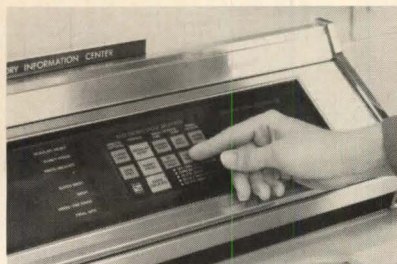
Touch-control washer (above) comes with a solid-state electronic control panel. Wash and rinse cycle durations and temperatures may be selected for different fabrics. Whirlpool, Benton Harbor, MI. Circle 211 on reader service card
