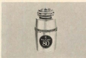
"Power 80" waste disposer (above), with automatic reversing action, is driven by a 1/2 hp motor. Unit features stainless-steel grind components and 360° swivel impellers, which assure jam-free operation. Elkay, Broadview, IL. Circle 205 on reader service card
