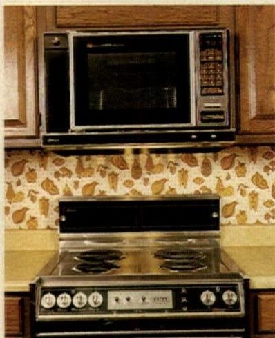
Space Saver II mounting provides an above-range exhaust ventilator, and accommodates a microwave oven. Prewired unit has 225 cfm double squirrel cage blowers. Ductless model is available. Dacor. Circle 222 on reader service card
