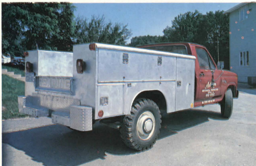
Lightweight aluminum service body is said to reduce truck fuel consumption and chassis wear. Reading Body Works. Circle 272 on reader service card
