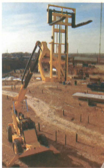
Extendo 88 high-lift , with 8' mast, can raise 2,500 lbs. 42 feet. Features include automatic leveling, four-wheel drive and 90° fork tilt. Attachments such as hydraulic winch, boom extension and special fork are available. Pettibone Corp. Circle 277 on reader service card
