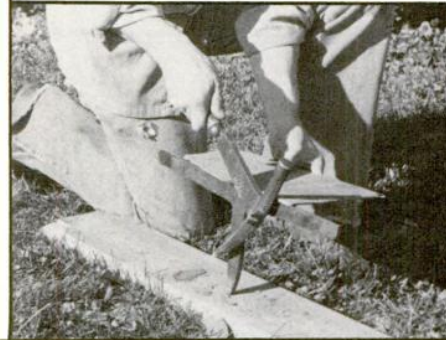
STAKE: T-bar (18 in. long) with the short arm pointed for driving into plank or scaffold. Long arm acts as rest for slate during punching and cutting operations, or as a straight edge.
