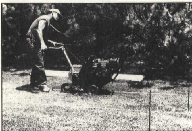
The gasoline-powered sod cutter pictured here is not just a fancy lawn mower, so you may want to hire a pro to operate it. (Note the stakes and cord used here to lay out the width of the path.)
