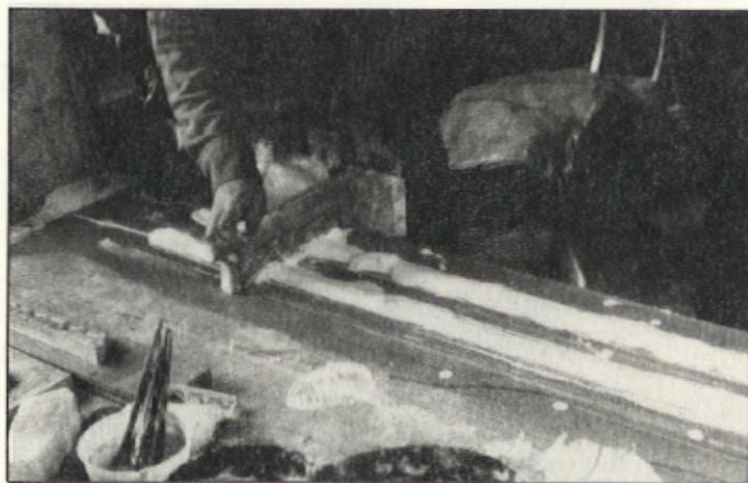
Step 4: Run the mould the full length of the piece, steadily and slowly, without stopping.
