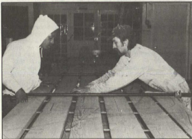
These two workmen are gluing up a backboard in Mike Pangia's shop. Note the identifying figures drawn across the boards — they're the real-life versions of the triangle and circle shown in the illustration on page 191.
