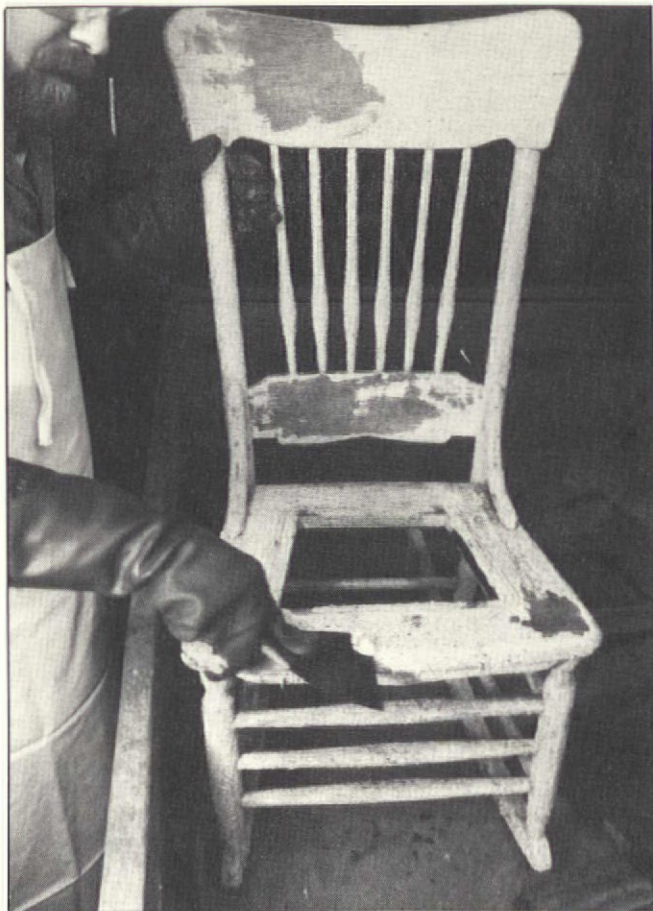
Scraping off the softened paint.
