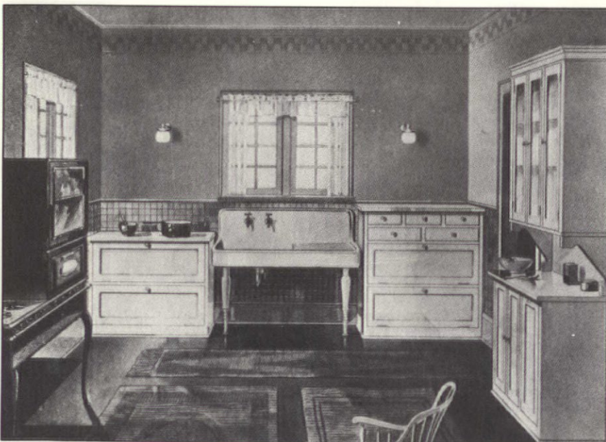
The illustration is from 1921, but the sink is comparatively old fashioned, being supported by legs. (Note, however, the built-in work surface in the right portion of the sink.)
