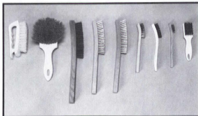
Nylon, plastic, brass, and steel brushes in various sizes are handy for getting into grooves and for final cleanup.
