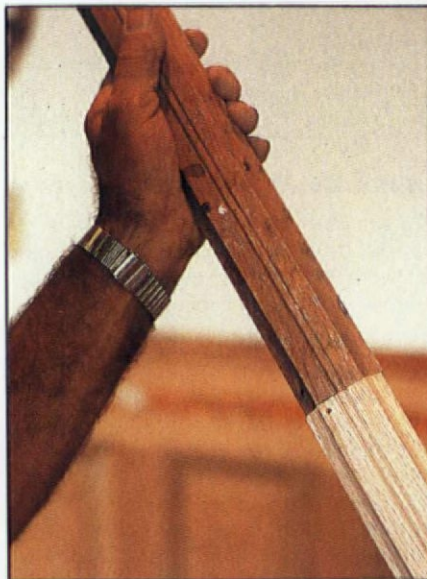
This moulding was duplicated by first cutting the coves with a router. The center bead was added with a Stanley moulding plane.
