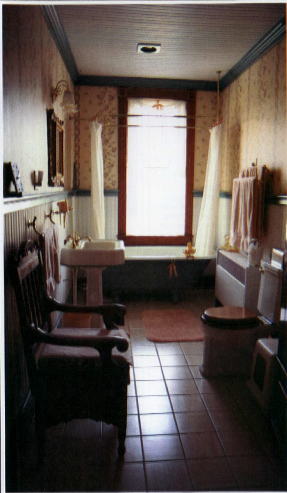
The May-West bathroom overcomes the feeling of a long and narrow room by regrouping the plumbing fixtures at one end and consolidating the dressing room furnishings such as the armoire and oak commode at the other end.
