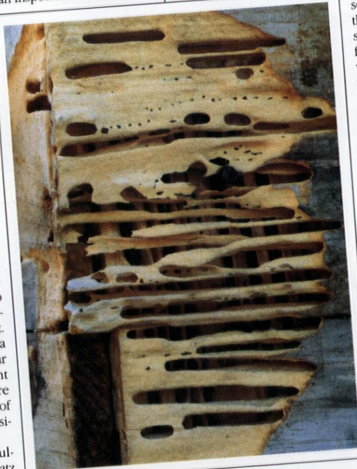
Clean, smooth-surfaced galleries chewed out of softwood sheathing — the nesting place of carpenter ants.
