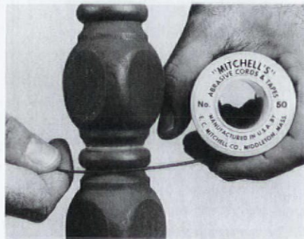
Large-width abrasive cords can be used with power tools as well as by hand.
