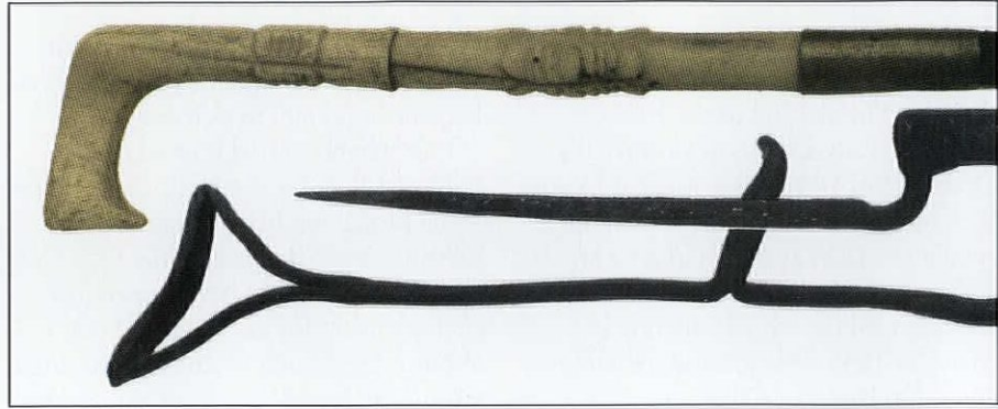
Our "Mystery Object" turns out to be a farrier's buttress for shoeing horses.
