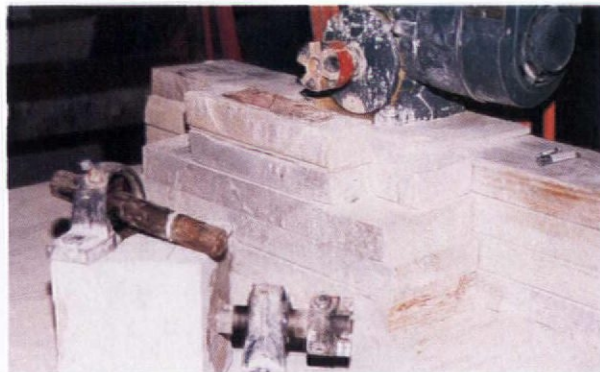
The motor/coupler assembly as well as the pillow blocks must be raised to the correct height (lumber works well) for the bit to cut properly.
