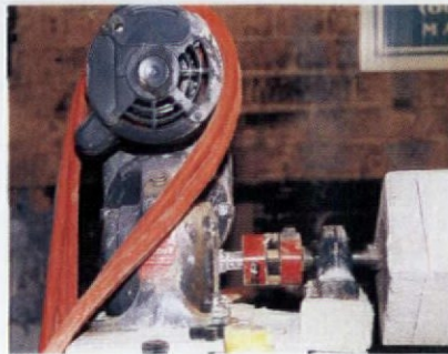
The drive train of the lathe: electric motor (at left in photo); right-angle reduction drive (under motor); Lovejoy coupling (center); steel shaft mounted in pillow block (right).
