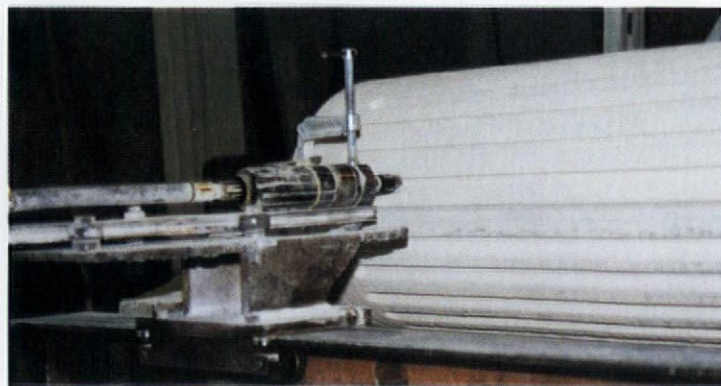
To create flutes, start with a saw kerf, then shape with a series of router bits ( \frac{1}{4} ", \frac{1}{2} " , \frac{3}{4} " ), and finish with a 1" bit.
