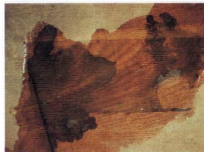
Water, not ink, put the blue puddle in this oak. Oxalic acid (top) started to bleach before the panel was completely wet (above).
