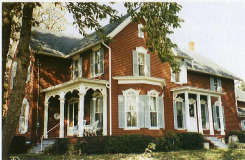
The Withrow's house, with its Italianate-style moulded window lintels with cutouts, is typical of comfortable middle-class homes of the mid-19th century.
