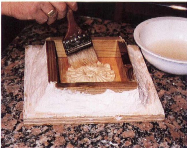
Plaster, clay, weights — anything handy — can hold the fence in place to make a flood mold. Once the joints are sealed, paint all surfaces with separating solution.
