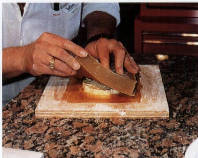
Work all the way around the model as you separate the mold from the bearing. If the model breaks free, release it from the mold by using slight pressure on the back.
