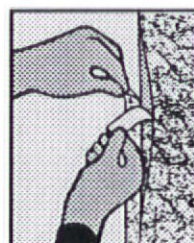
11. Remove mat strips on both sides of cut.
