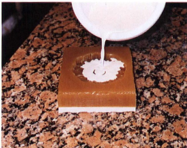
After a fresh coat of separating solution, the mold is ready for pouring a casting. Watch for heat buildup in the plaster, and unmold as soon as it's set.
