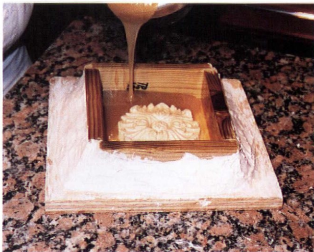
Starting at one end of the bearing, pour the molten glue between the model and the fence. Avoid trapping bubbles. Puddle leftover glue on a clean surface for recycling later.
