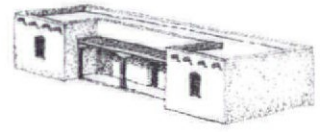
Flat roof with parapet and supporting vigas , or round timber beams.
