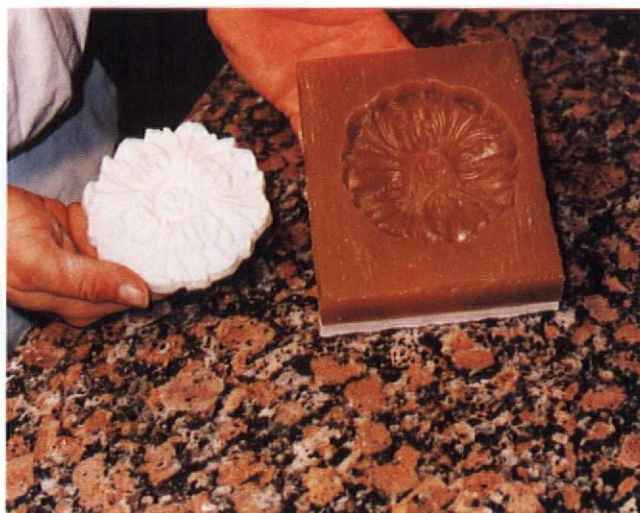
The finished cast shows all the details of the original. Check the mold face for soft spots — the result of heat, moisture, or bacterial attack — before starting another cycle.
