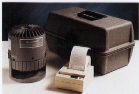
Both the continuous radon tracker (left) and E-Perm detector (right) offer short-term tests for quick results, and long-term for average levels.
