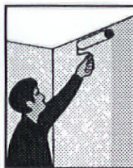
2. Apply saturant to area to be covered.
