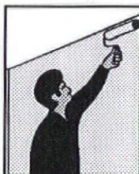
12. Apply 2nd coat of saturant (include seam)
