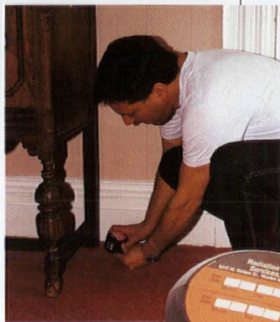
Short-term testing is cheap and easy, and usually the only option for homebuyers, but determines radon levels only for the days it is set. Tests in winter give the highest readings.
