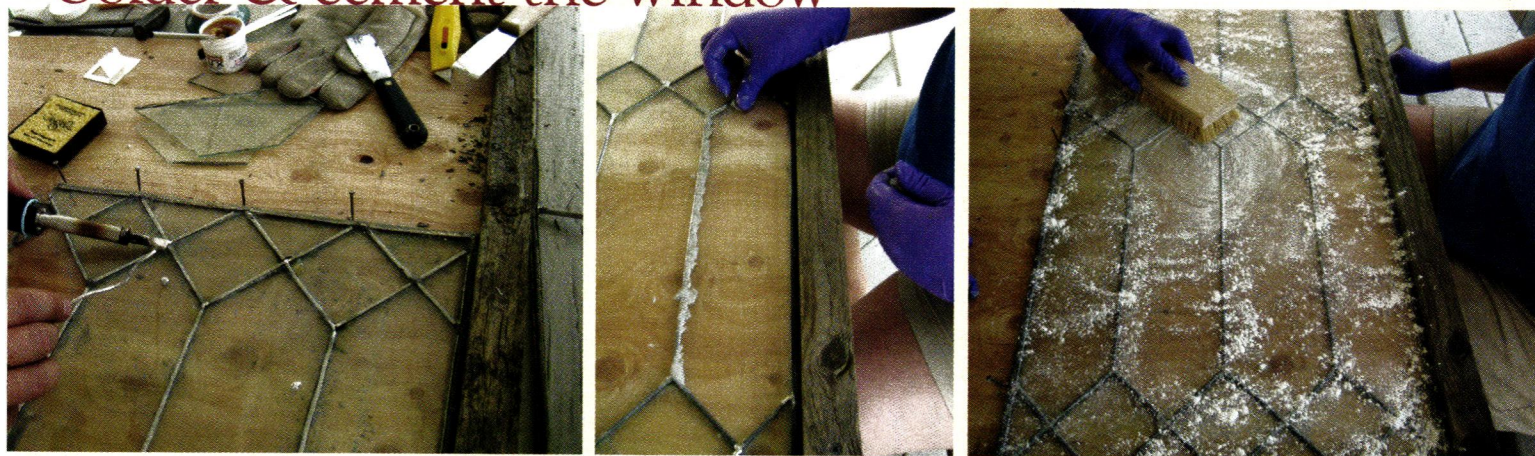
LEFT TO RIGHT: Brush flux on joints, then melt solder into them with a hot soldering iron. Press glazing putty into spaces between came and glass, then remove excess putty, sprinkle the window with whiting, and brush it with a natural-bristle brush to create a dark patina.
