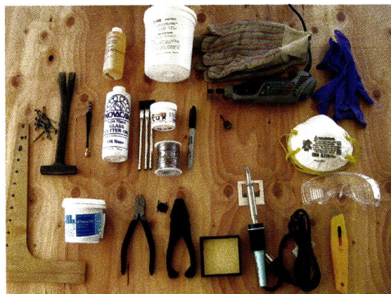
Necessary tools include a rotary tool, soldering gun, breaker pliers, and safety equipment.
