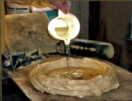
FORM the resulting putty into a donut shape on the worktable; pour water in the reservoir.
