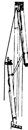
A cross section of window shown opposite. Shades adjustable to any position. No obstruction to air. No flapping, no tearing.
