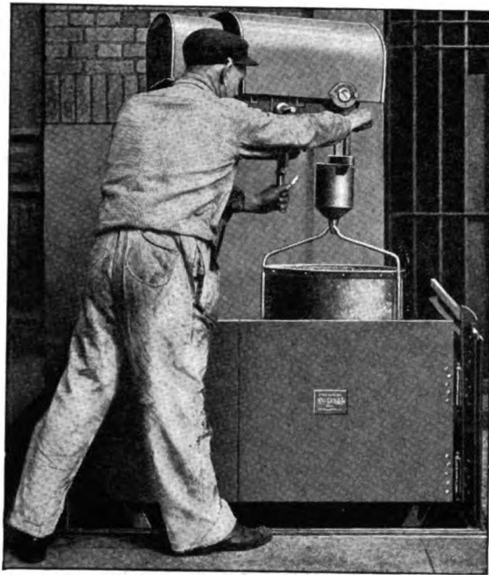
G&G Model E electrically operated hoist in use at R. H. Macy Co.'s new warehouse, New York City. Robert D. Kohn, Architect.
