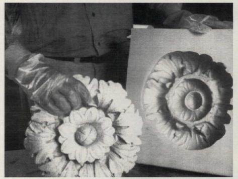
This rosette reproduction, with all the detail and contours of the original, was made from SYNAIR's "Por-A-Mold" products. Also available are unique powders and fillers that can be used to recreate special textures, colors, and weig
