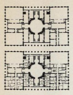
The top plan shows the original layout of the Statehouse's second floor. The bottom plan is the same floor after years of subdivision and filling in of corridors and light courts. The results were mechanically inefficient and very unsafe.
