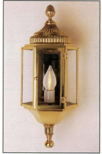
▲ Fixture 1002. Brass wall lantern, 12" x 27", 3 candelabra base incandescent sockets up to 60 watts each. Alternative glass, finish and lamping available.
