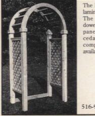
The DELUXE ARBOR consists of a laminated, clear, inland red cedar arch. The connecting spindles are 2x2 doweled red cedar. The two 2'x4' lattice panels are made of northern white cedar. Four 4x4x8 red cedar posts complete the set. These arbors are available in 3', 31/2', 4', 5', 6' and 8' wide.
