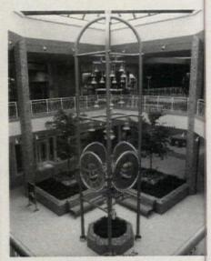
The Masonville Mall in London, Ontario, keeps up with the times with this tubular steel bell tower from ELDER-HORST BELLS, which has a custom designed four-face clock. A computer control panel operates individual electromagnetic clappers that enable the 19 tuned bronze carillon bells to play various tunes. Write in No. 2100
