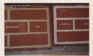
Epochrome S, distributed by Cathedral Stone Products, is designed to blend new pointing mortar with that of the rest of the building. In the test panels shown here, raw untreated mortar is on the right. On the left, the mortar has been grayed, to create a patina that simulates the visual effects of aging. Write in No. 9580
