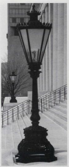
For the Ohio State Capitol building, HISTORICAL ARTS & CASTING supplied ornate gas lamps that employ an electric-ignition and flame-sensing system. Write in No. 1210
