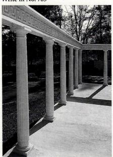
Manor Style's load-bearing, fluted fiberglasscomposite columns and custom-fabricated PVC Greek Key-patterned beam adorn this
