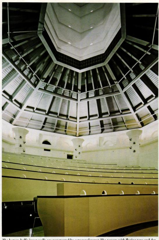
The lecture hall's inner walls are punctuated by octagonal turret-like towers with flaring tops and dotted with eyeball-like air-conditioning registers. The faceted ceiling slopes up toward an oculus opening into the cupola above, making a dramatic focal point. The details of the exposed steel framing were "fussed over" and the building's systems were exposed for instructional value.
