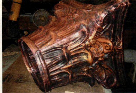
Heather & Little fabricated this copper capital.
