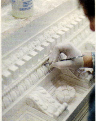
A Foster Reeve artisan touches up every final detail of this custom ornamental entablature prior to installation.
