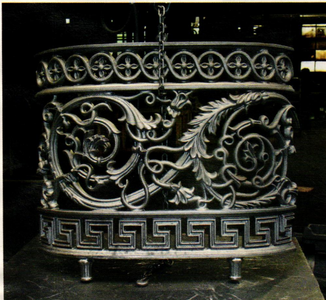
This curved section of fence was cast by O. K. Foundry to match the curbing of the Palmer fence at Hollywood Cemetery in Richmond, VA.
