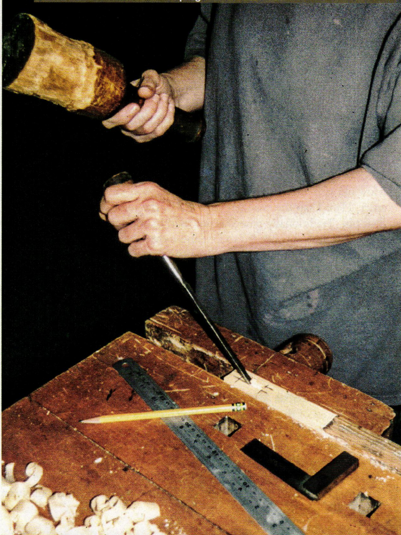
Final shaping of the dutchman.
