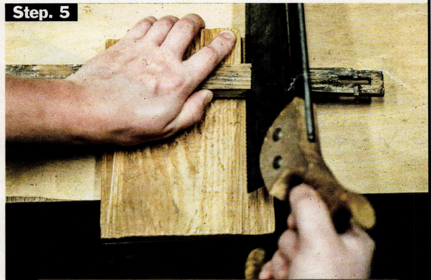
The stile socket is shaped with traditional woodworking tools.
