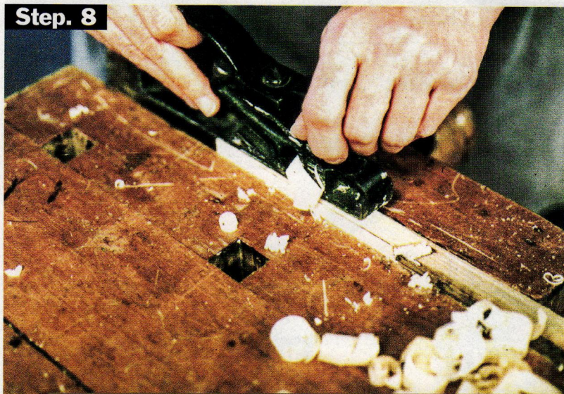
Final shaping of the dutchman.
