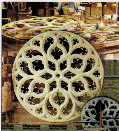
Bovard Studio custom wood window frames such as this one; shown in various stages of installation at the 1st Presbyterian Church in Fort Smith, Arkansas.
