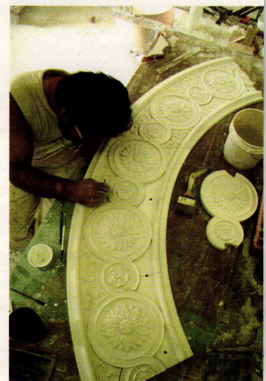
A craftsman at Felber Ornemental is shown completing a custom "guilloche" model.
