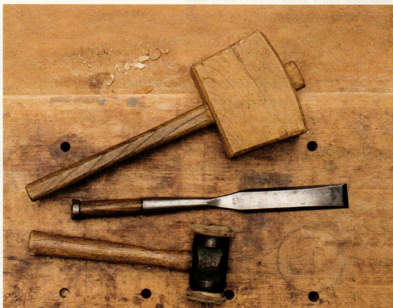
BELOW: The author encourages his audience to be mindful that since timber framing uses large dimensional wood (greater than 5 by 5 inches) that a few tools should be used to “bring the tools to the work piece rather than the other way around.”
