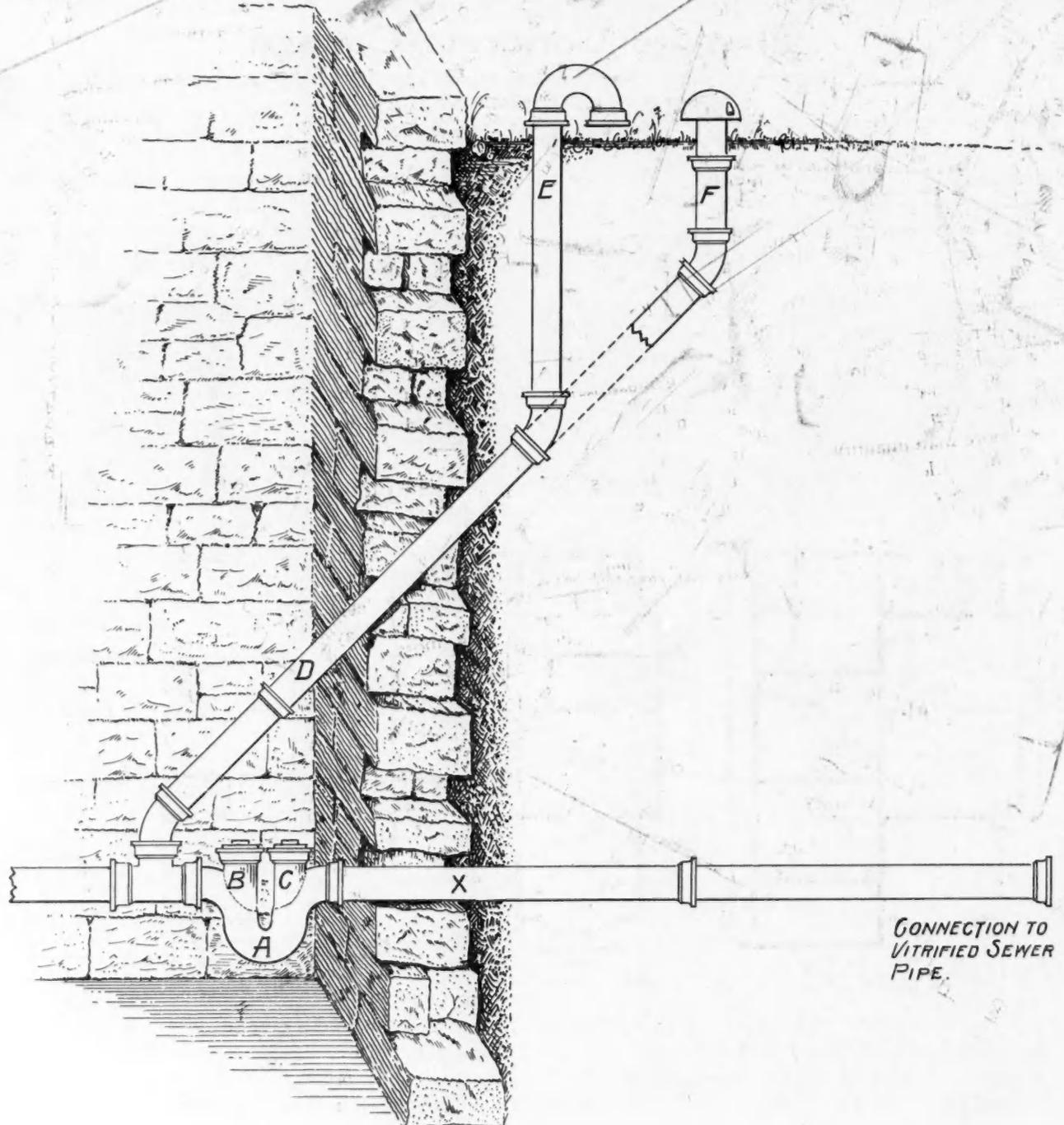
which ordinarily accompanies water. The pipe should be laid to grade, or a fall of one foot in forty feet. Care should be exercised to allow a large enough opening in the wall where the pipes pass through it, and especially over them, to allow for settling of the wall without touching them.
