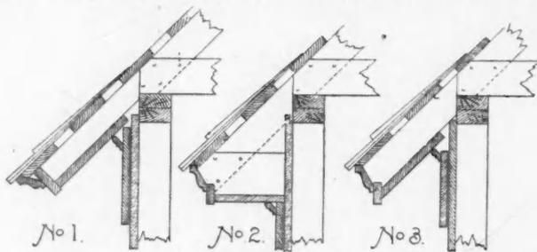
at the rafters square, but if it is a box cornice like No. 2, then the crown mould should set plumb. A cornice like No. 3 will not work well where there are gables, because the crown mould will not member with that of the gable.
