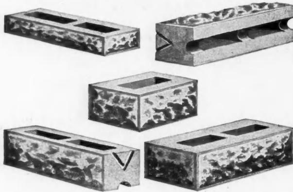
The main object was the making of a block that would be damp proof and frost proof. This was attained by the construction of a block that has double air spaces, one of which is vertical, as in the ordinary hollow block, while the other is horizontal, making the air space continuous in a wall made of these blocks.
