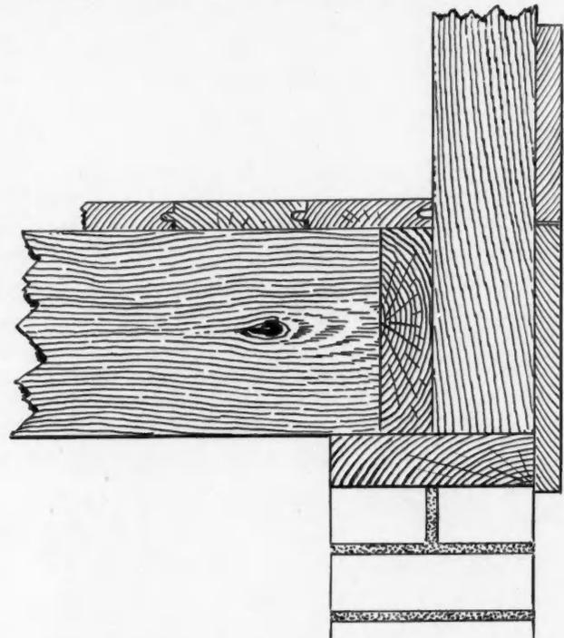
made this way are, first, you get the full strength of the studding; second, less work cutting same; third, it makes a tight job all around, so wind, mice or rats cannot get into the house or between the partitions; fourth, it is easier to lay floor, as you have no studding to cut around. This may be new to some one.
