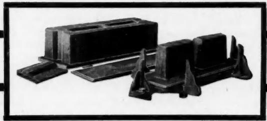
The Clipper Block Machines are simple, durable, light, strong, accurate, and will produce a great variety of shapes and sizes in hollow blocks, veneering blocks, chimney blocks, pier blocks, circular blocks.
