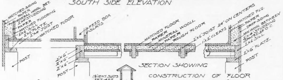
SECTION SHOWING CONSTRUCTION OF FLOOR
