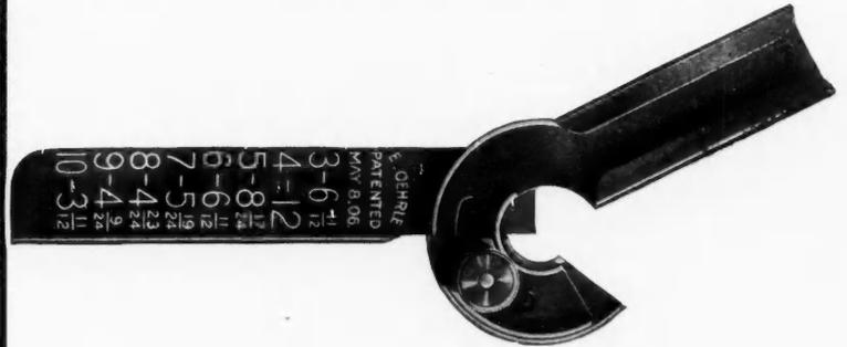
jacks. Figures are stamped on it showing how it may be used for polygon cuts and how to obtain rafters for all polygon roofs of from three to ten sides.
