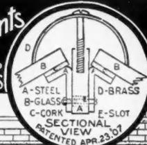
Handiest, Strongest and Most Practical Bar on the Market. Long Life—nothing to rot out. Glass Bedded on Spanish Cork, preventing cracking or Crushing of glass. No putty, yet ABSOLUTELY WATER AND DUST PROOF.
