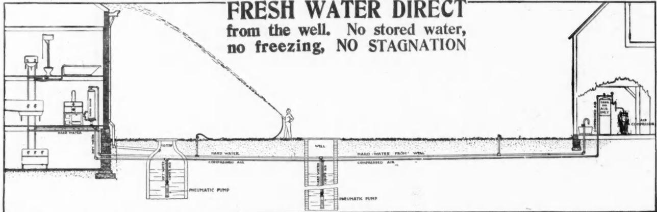
The PERRY PNEUMATIC WATER SYSTEM furnishes water at any given pressure at the faucets by means of compressed air. Power and air compressor operate only occasionally to keep air reservoir charged. This stored air is used, and the Perry Pneumatic Pump operates only when water is drawn. Air may be piped to pumps in widely separated wells. Well and cistern water may be obtained with one air reservoir, as illustration shows.
